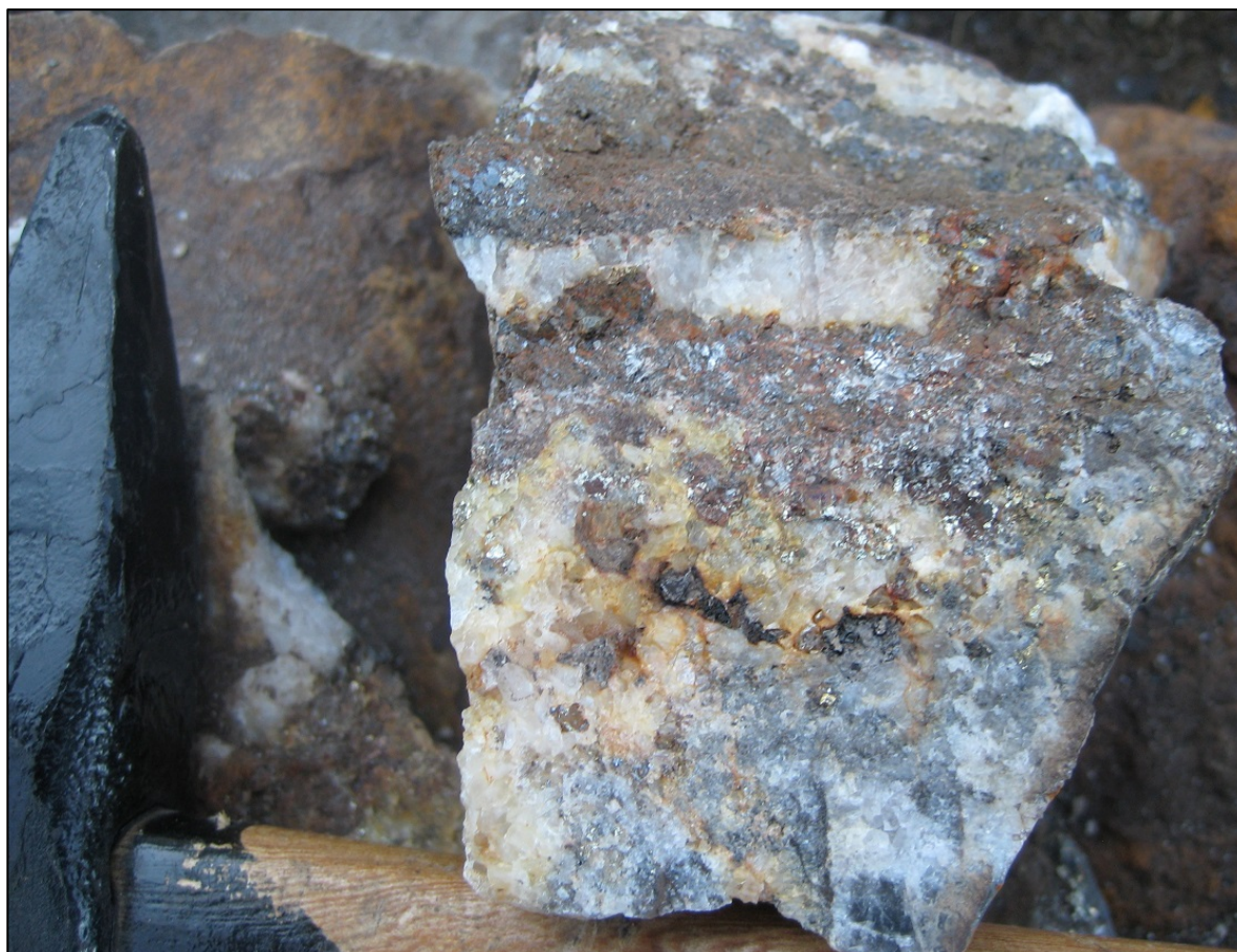
Figure 3-7: Massive sulphide (partially oxidised) with quartz from the Sentazon mine, Cerro Sur
