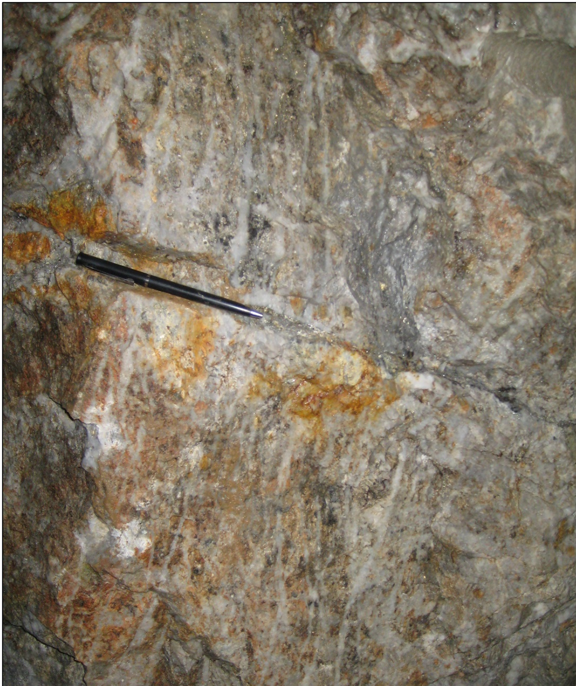
Figure 2-10: Intrusive breccia in an underground exposure from the Gold Block overprinted by steeply dipping quartz veins and a later shallowly dipping quartz-pyrite-arsenopyrite vein
